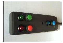
In case of stopping the car on the SS system is sending the warning signal to the car unit. The lamps in manipulator panel (Green and Red) start blinking. That means that operator of RCC see the car standing on the SS and expect to have the information from the crew. Within 1 minute from stopping over the Special Stage the driver or the pilot should press the proper button to clarify the situation.
